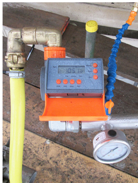
Timer to programme intermittent cleaning cycles and pressure gauge.
